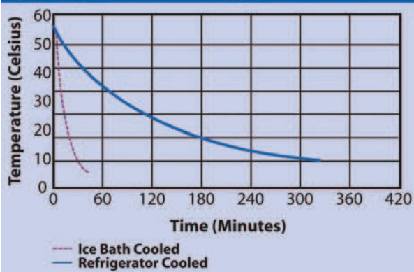
Figure 5. Cooling Rates of Serum in ice baths or refrigerator.
