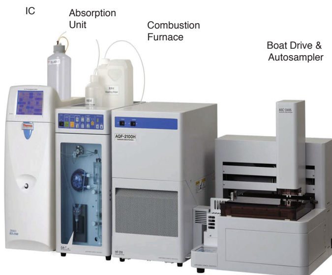
FIGURE 2. Combustion ion chromatograph.
