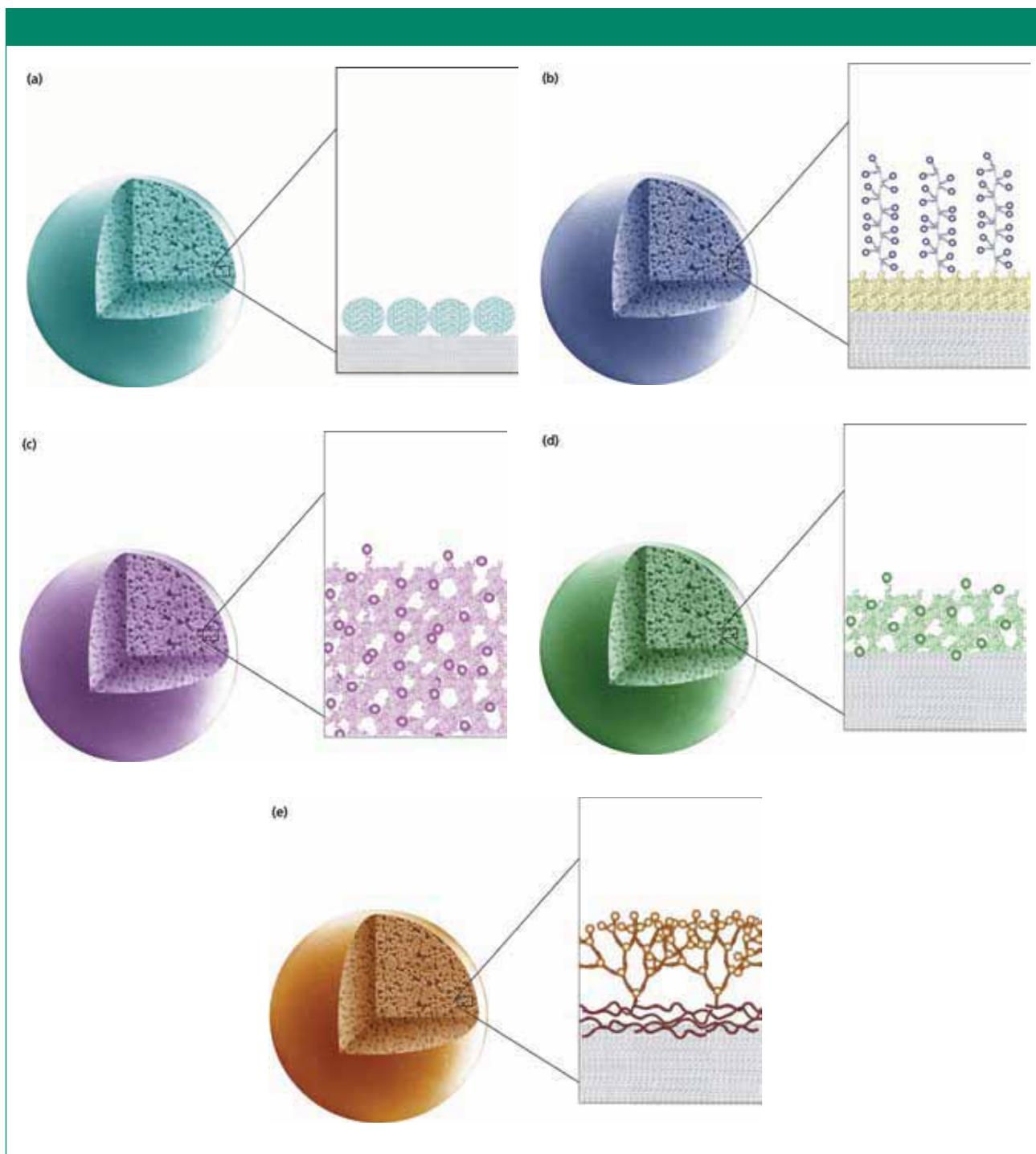
**Figure 1:** Ion chromatography stationary-phase architectures most widely used in recently introduced phases: (a) electrostatic agglomerated ultrawide-pore substrates, (b) polymer-grafted film on porous substrates, (c) chemically derivatized polymeric substrates, (d) polymer-encapsulated substrates, and (e) step-growth polymers on polymeric substrates.
