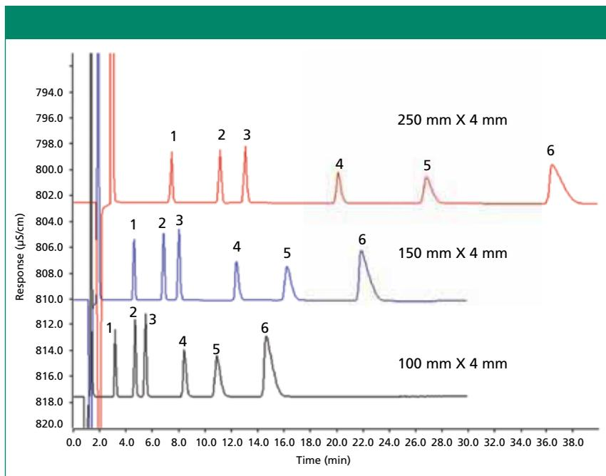
**Figure 6:** Ion chromatography separation of alkali metals and alkaline earths. Column: Metrosep C6, 4 mm; eluent: 1.7 mM nitric acid, 1.7 mM dipicolinic acid; flow rate: 0.9 mL/min; temperature: ambient; detection: conductivity. Peaks: 1 = lithium, 2 = sodium, 3 = ammonium, 4 = potassium, 5 = magnesium, 6 = calcium.
