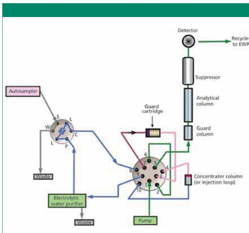
**Figure 4:** Example analytical setup for use of in-line sample preparation followed by preconcentration of the target analytes. The water for the loading pump should be cleaned using an electrolytic water purifier for minimal background.
