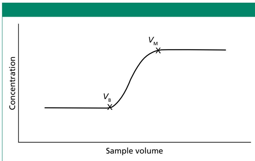
**Figure 2:** A typical breakthrough curve for a sample preparation cartridge.
