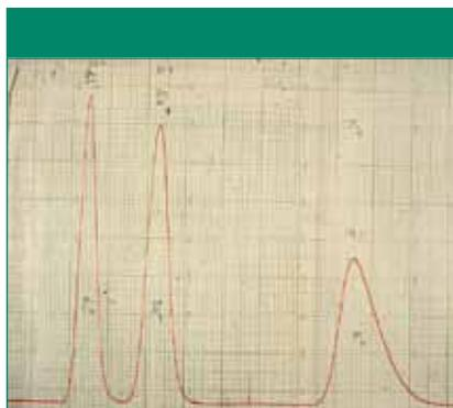
**Figure 2:** The first chromatogram using eluent suppression and conductometric detection. The sample injected was 0.1 mL of a mixture of LiCl, NaCl, and KCl, 0.01 M of each. The eluent was 0.02 M HCl. From author’s laboratory notebook, dated November 9, 1971.
