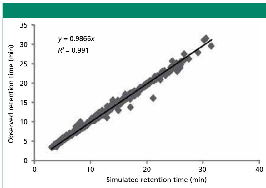
**Figure 6:** Correlation of experimental and simulated retention times for 24 anions and 13 cations on Dionex AS11 HC, AS16, AS19, CS12A, and CS16 columns for four 5-step complex eluent profiles.
