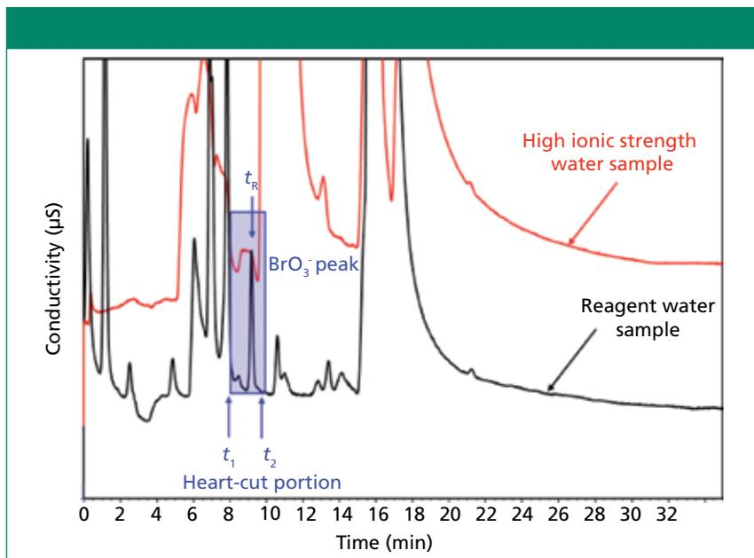
**Figure 5:** First-dimension analysis of a bromate peak in reagent water and high ionic strength water. The bromate concentration is 15 µg/L. The bromate retention time ( $t_R$ ) is 9.2 min. The start of the cut window ( $t_1$ ) is 8.0 min and the end of the cut window ( $t_2$ ) is 9.8 min. Column: 25 cm × 0.4 cm IonPac AS19; eluent: 10 mM KOH, step changed to 65 mM KOH following the elution of bromate at 1.0 mL/min; injection volume: 1.0 mL. (Courtesy of Thermo Fisher Scientific.)
