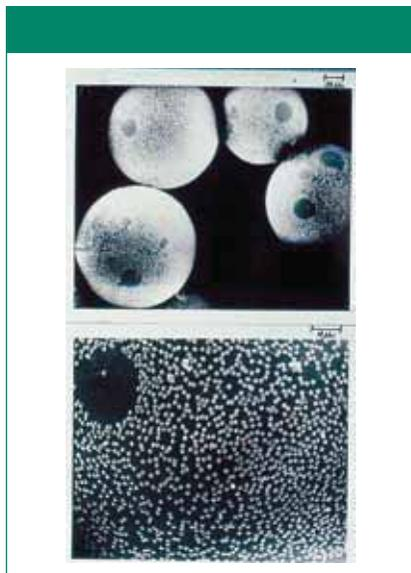
**Figure 3:** (Bottom) Colloidal anion-exchange particles (about 300 nm in diameter) on surface-sulfonated styrene-DVB particles (about 50  $\mu\text{m}$  in diameter) (top).
