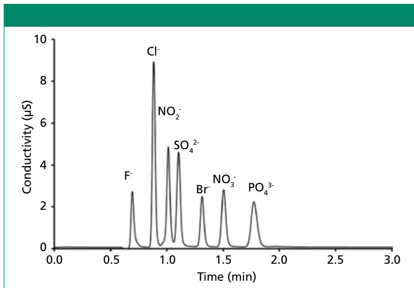
**Figure 2:** Fast separation of seven common anions on an IonPac AS18 capillary column (150 mm × 0.4 mm) packed with 4- $\mu$ m particles. Eluent: 35 mM OH<sup>-</sup> with a flow rate of 25  $\mu$ L/min; operating pressure = 3480 psi. Suppressed conductivity detection. Adapted from reference 16.
