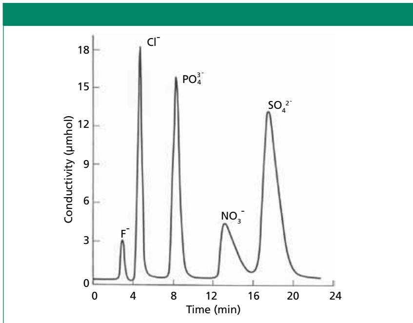
**Figure 4:** Status of anion IC using carbonate eluent, circa 1974.
