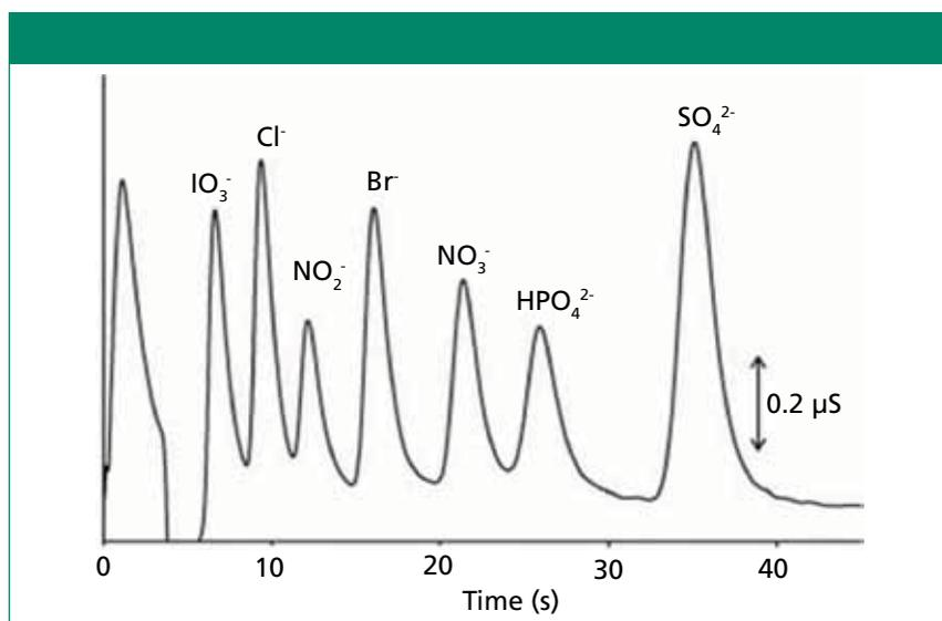
**Figure 3:** Ultrafast separation of seven common anions on very short column (1.3 cm × 0.46 cm) with suppressed conductivity detection. Column: Cationic surfactant (didodecylidimethylammonium bromide) coated Extend-C18 column; flow rate: 2.0 mL/min; particle size: 1.8  $\mu$ m; eluent: 2.5 mM 4-hydroxybenzoic acid (pH 10.1). Adapted from reference 20.
