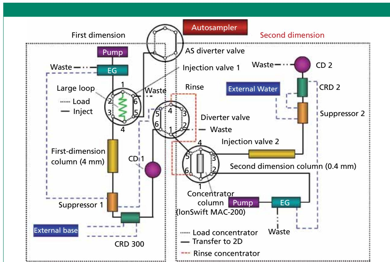
**Figure 3:** Two-dimensional ion chromatography instrumental setup.
