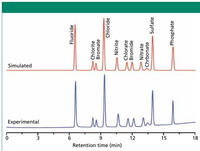
**Figure 5:** Simulated and experimental separations on a Dionex AS19 column under a three-step gradient profile consisting of: 3.75 mM KOH for 0.8 min, 3.75 to 33.75 mM KOH for 10 min, followed by 33.75 to 99.75 mM KOH for 4 min at 1 mL/min at 30 °C.
