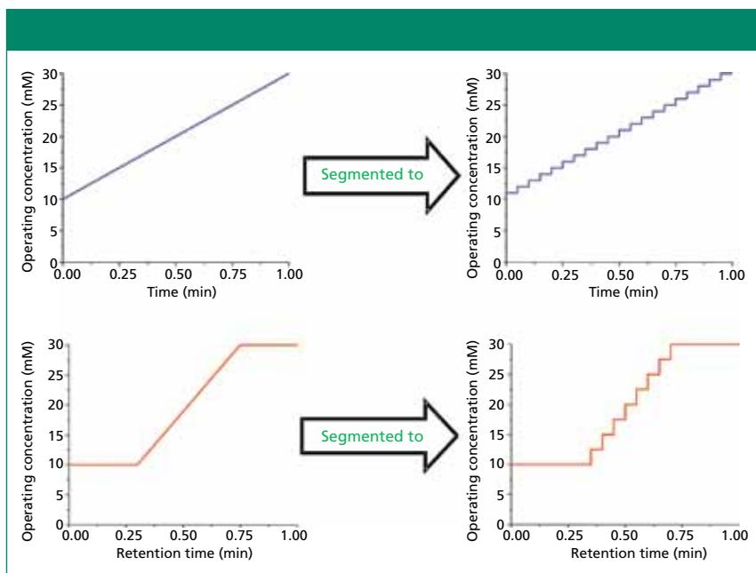
**Figure 3:** Schematic overview of segmenting gradients and multistep profiles to isocratic segments.
