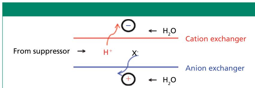
**Figure 2:** Basic schematic for the charge detector.
