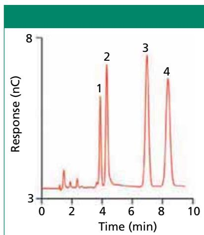
**Figure 5:** Determination of carbohydrates by IC: 1 = glucose, 2 = fructose, 3 = lactose (internal standard), and 4 = sucrose. Adapted from reference 43 with permission.
