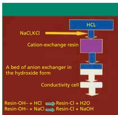
**Figure 1:** Workflow devised in 1971 using a “stripper” column between the separator column and the conductivity cell, as applied to the separation of the alkali metals on a cation-exchange resin using hydrochloric acid as the eluent.
