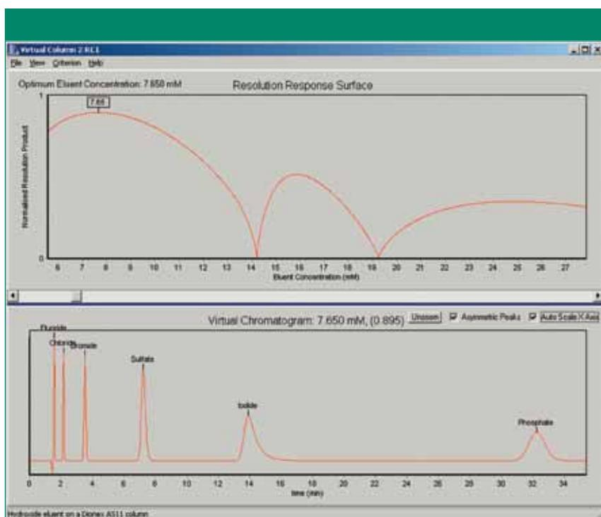
**Figure 4:** Screen display from Virtual Column software for isocratic separations.
