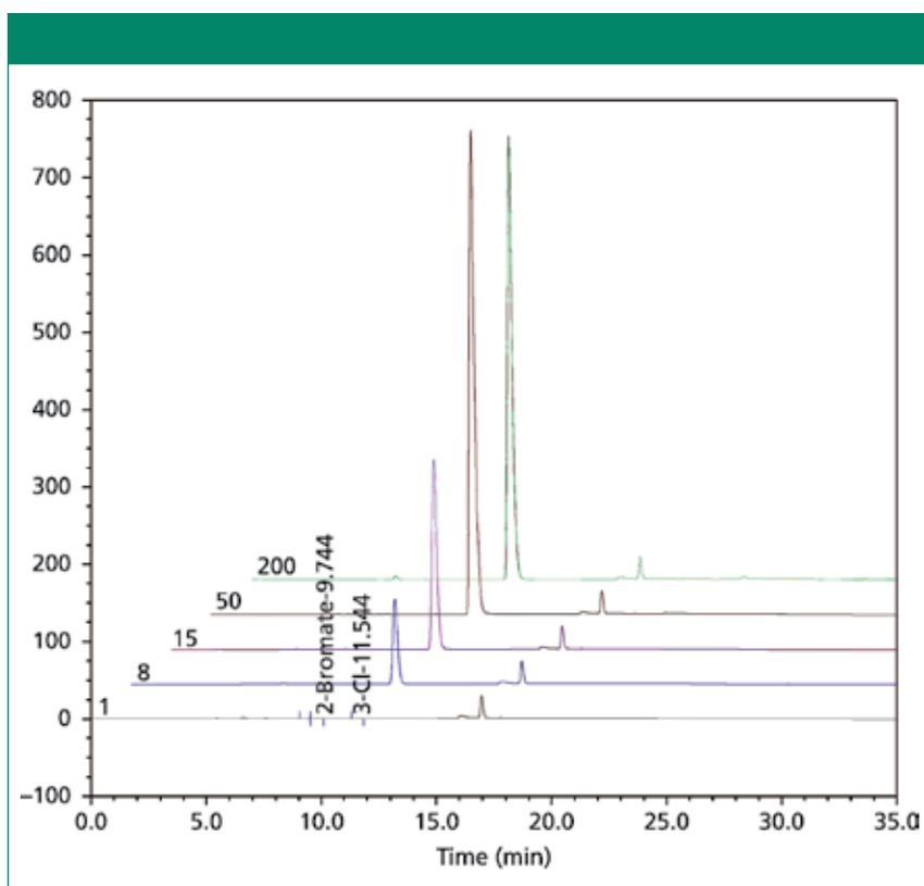
**Figure 5:** Comparison of lifetime chromatograms for 10 ppb bromate in 300 ppm chloride using sample preparation. Columns: IonPac AG24/AS24 (250 mm × 2 mm); eluent: 15–50 mM KOH gradient; flow rate: 0.3 mL/min; suppressor: ASRS 300 (2 mm); concentrator: TAC-ULP1; injection volume: 500  $\mu$ L; sample preparation: InGuard Ag/InGuard H; sample loading: deionized water, 0.5 mL/min, 6 min.
