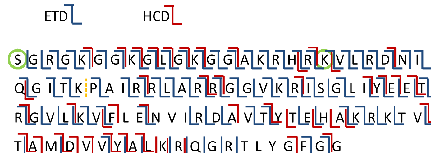
FIGURE 3. Histone H4 (12.3 kDa) HCD (top trace) and ETD (bottom trace) spectra and identification and annotation using Thermo Scientific ProSightPC software
