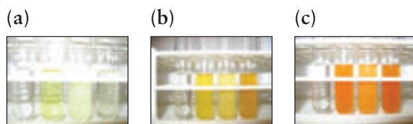
Figure 1: Anti-dandruff shampoo samples after the addition of potassium iodide solution. (a) immediately after addition, (b) 5 minutes after addition (c) 10 minutes after addition.
