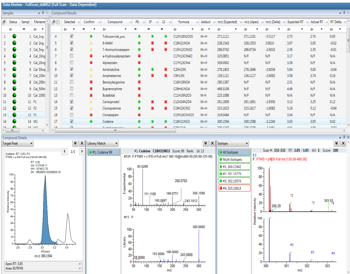
FIGURE 5. ToxFinder data review page: Compound results table with compound chromatogram, library search and isotopic match results.
