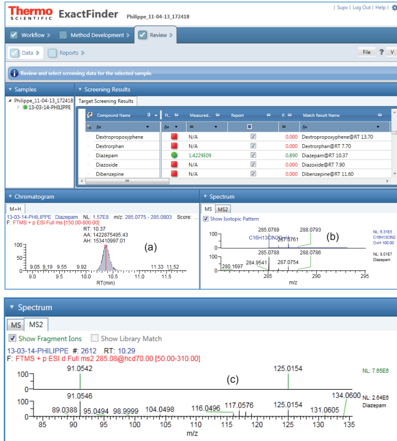
FIGURE 5. ExactFinder results page showing XIC chromatogram for Diazepam reconstructed with 5 ppm mass window (a), isotopic pattern (b) and fragment ion confirmation (c).
