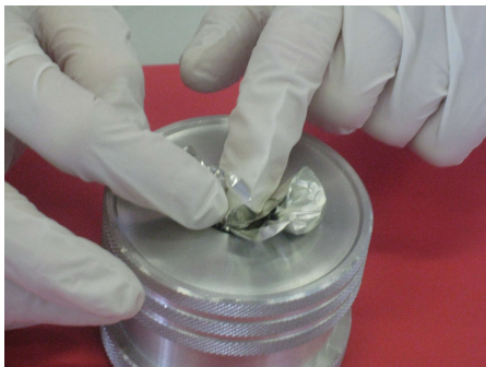
The tin disk including the sample is closed by hand.
