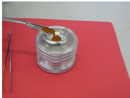
Using a spatula, introduce the sample into the capsule.
