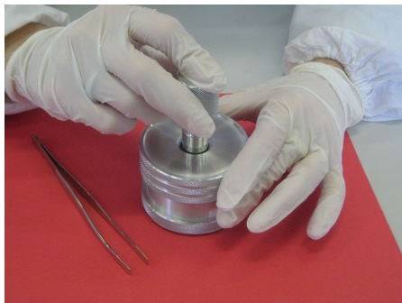
Using the cylindrical tool, press the disk and make it enter the cavity.
