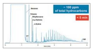
Figure 9: Real water extract chromatogram
