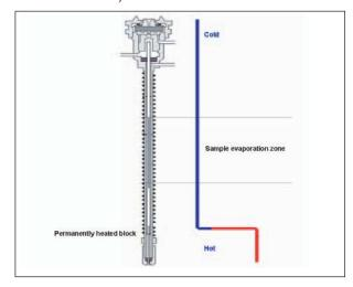
Figure 3: PTV inlet temperature profile
