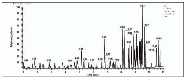
Figure 2: Total ion chromatogram of 20 µg/L method validation standard
