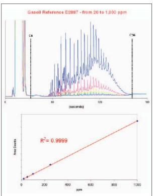
Figure 6: Linearity Test: 5 overlaid chromatograms and linear curve
