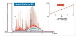
Figure 6: Linearity Test: 5 overlaid chromatograms and linear curve.
