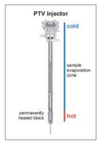
Figure 2: PTV inlet temperature profile.
