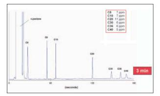
Figure 4: Standard chromatogram nC6-nC40
