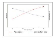
Graph 1: Pump speed vs Absorbance and Stabilization Time
