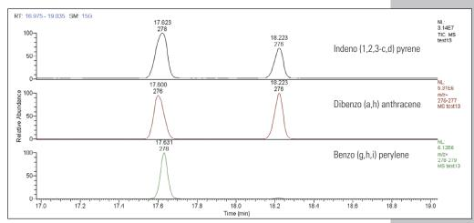
Figure 7: The transferline design of the mass spectrometer reduces band broadening of the late eluting polynuclear aromatics (PNAs): indeno (1,2,3-c,d) pyrene, dibenzo (a,h) anthracene, and benzo (g,h,i) perylene
