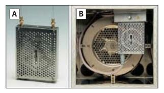
Figure 1: UFM column module (A) and its housing in a TRACE GC Ultra oven (B).
