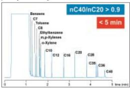
Figure 3: Standard chromatogram nC7-nC40.
