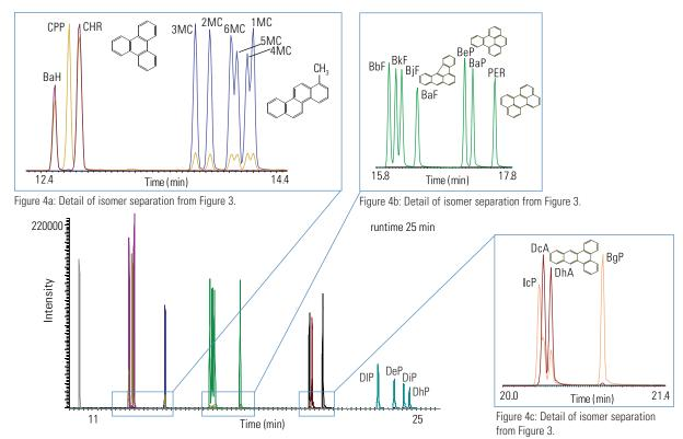
Figure 4: Fast GC separation with zoom.
