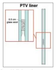
Figure 8: PTV liner model with glass wool.
