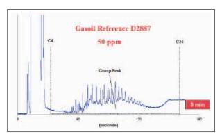
Figure 7: Gasoil Reference D2887 analysis
