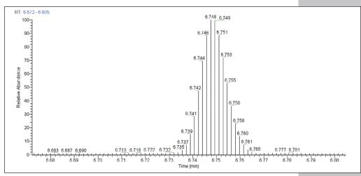
Figure 6: 20 scans across 1.8 second wide DFTPP peak, demonstrating good peak characterization
