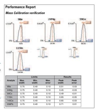
Figure 1 - Performance Report Results for Mass Calibration and Resolution Checks
