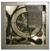
Figure 2: UFM column module(A) and its housing in a TRACE GC Ultra oven (B).
