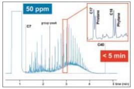
Figure 5: Gasoil Reference Mix, 50 ppm.
